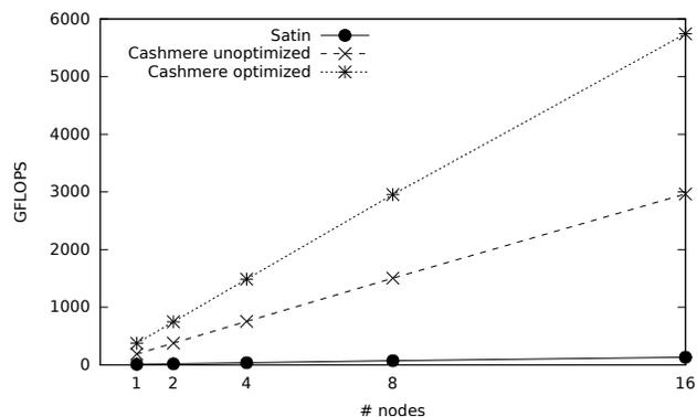
Figure 14. Absolute performance of N-body up to 16 GTX480 GPUs.
