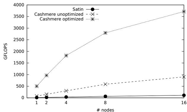
Figure 10. Absolute performance of Matrix Multiplication up to 16 GTX480 GPUs.
