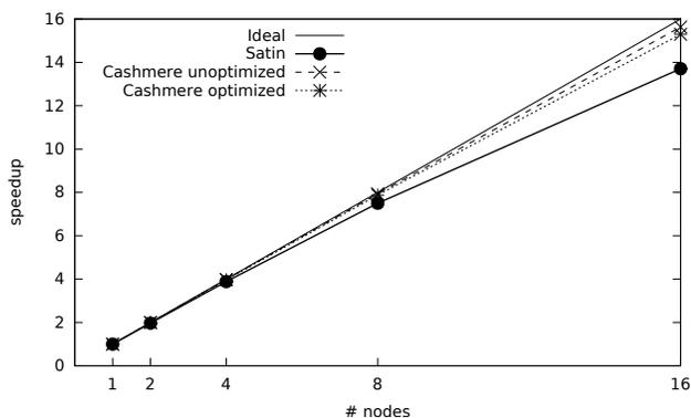
Figure 13. Scalability of N-body up to 16 GTX480 GPUs.
