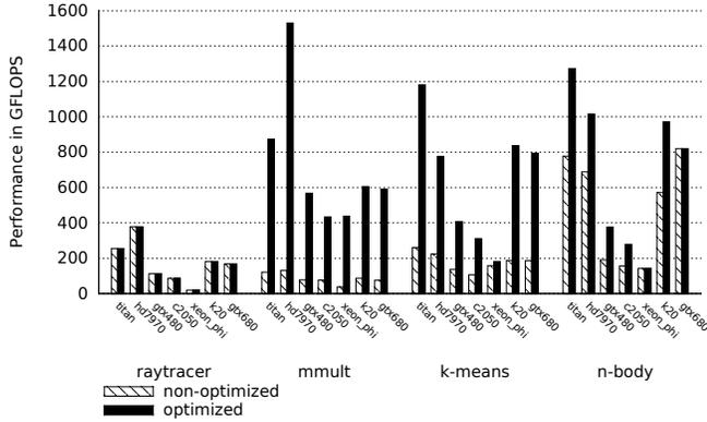
Figure 6. The performance of the kernels for the applications for the unoptimized version and the optimized version.
