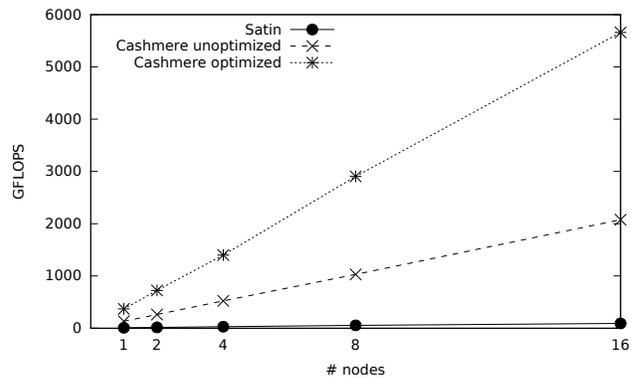
Figure 12. Absolute performance of K-means up to 16 GTX480 GPUs.
