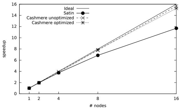
Figure 11. Scalability of K-means up to 16 GTX480 GPUs.
