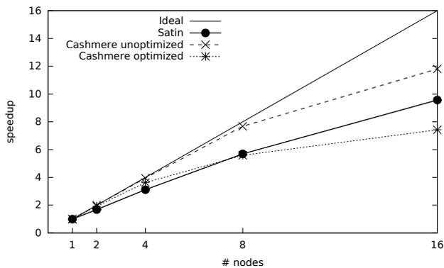
Figure 9. Scalability of Matrix Multiplication up to 16 GTX480 GPUs.
