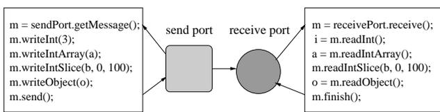
Figure 2: Send ports and receive ports.
