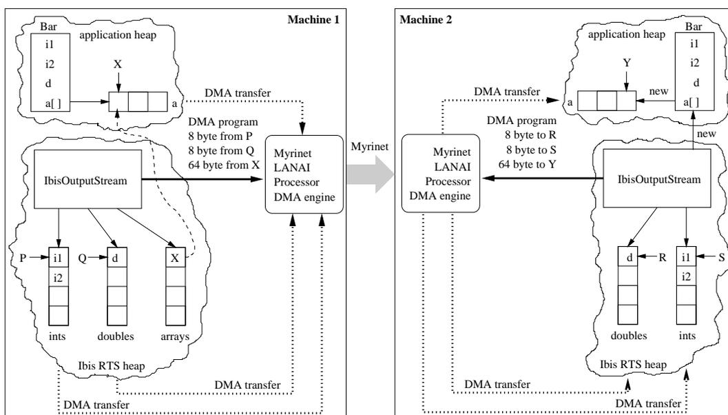
Figure 8: Low-level diagram of zero copy data transfers with the Ibis implementation on Myrinet.
